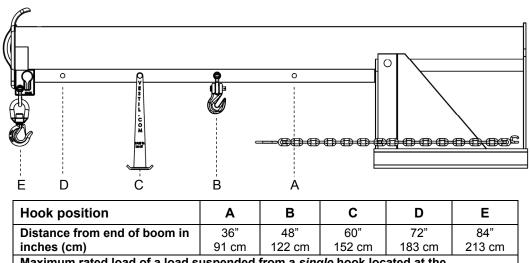
Maximum rated load of a load suspended from a single hook located at the corresponding "Hook position" 4000 lb. 3750 lb. 3500 lb. 3250 lb. 3000 lb. LM-1NT-4k 1820 kg 1590 kg 1363 kg 1705 kg 1477 kg 5000 lb. 4500 lb. 4000 lb. 3500 lb. 6000 lb. LM-1NT-6k 2045 kg 2727 kg 2272 kg 1820 kg 1590 kg 6000 lb. 5300 lb. 8000 lb. 6650 lb. 4850 lb. LM-1NT-8k 3636 kg 3022 kg 2727 kg 2409 kg 2205 kg
