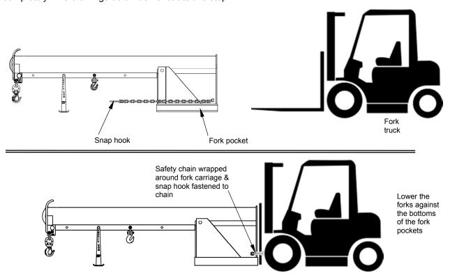
Securely connect the boom to the carriage of the forklift with the safety chain.
