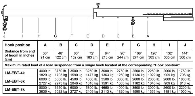
The center of gravity of the boom changes as boom length changes. As shown in the diagram below, the horizontal center of gravity may be located at any point from RHCG to EHCG:
