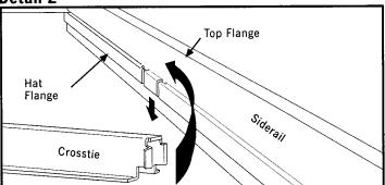
Determine whether shelves will be used for 25 PSF or 50 PSF capacity. 25 PSF shelves ship with (5) crossties each; 50 PSF shelves ship with (9) crossties. 25 PSF shelves use crossties in locations 1,3,5,7, and 9. 50 PSF shelves use crossties in all 9 locations. (See Finished Assembly detail) Place crosstie between assembled rails as shown in Figure 2. Rotate the crosstie so it is between the top flange and hat flange of the siderails as
