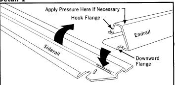
Place endrails and siderails out as shown in Figure 1. Take a siderail and engage downward flange of both endrails into slots as shown in Detail 1. Rotate the siderail so that the hook flanges engage corresponding slots in siderail. It may be necessary to squeeze or apply pressure to the top of the endrail to engage the hook in the slot. Repeat for other siderail.
