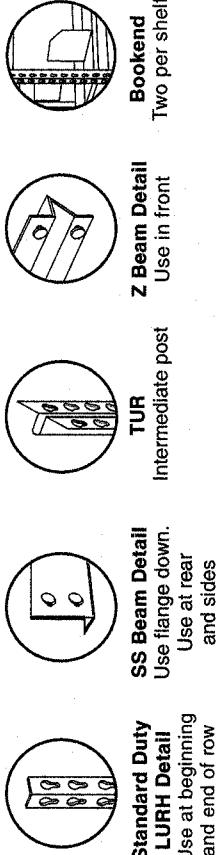
**Step 1** Assemble left side of unit by attaching shorter SS beam (flange down) to two LURH posts at the 2nd and 3rd rivet hole location (working from the ground level up) and at the very top rivet hole location. An additional shorter SS beam will be placed in the middle, in Step 5.
