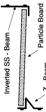
Note: Particle board is 3/8" lower at rear to keep files in place.
