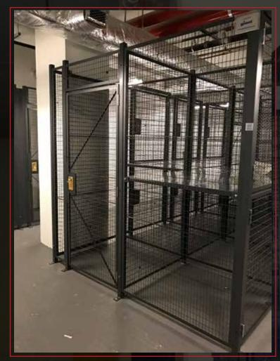
When larger cages or key locks are required, we recommend our modular partition system. Panels bolt directly to support posts. Standard 3/8" wedge anchors hold partition firmly in place. Baseplates welded on posts allow direct floor anchoring.
