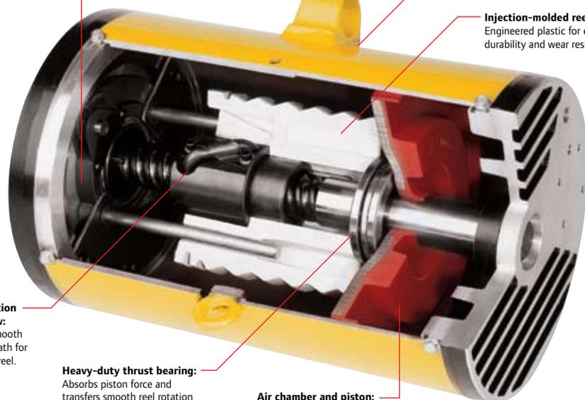
**Anti-friction ball screw:** Creates smooth rotation path for the cable reel.
