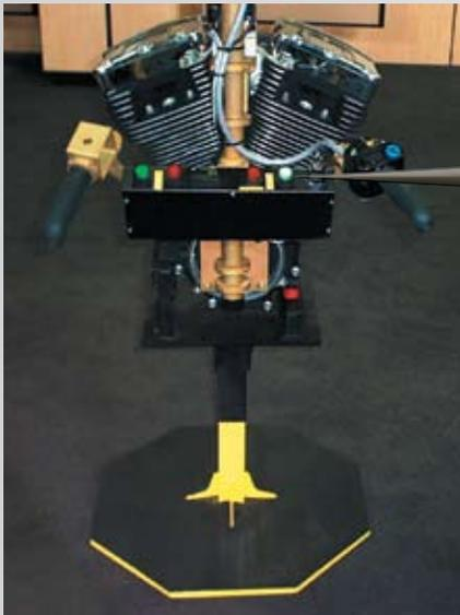
The engine-handling device shown uses the unique features of the IntelIFT balancer. Features include: auto clamp, interlock, up control disable, weight sensing with automatic alarm, and keyed lockout.
