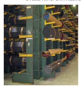
Cantilever rack allows storage shelves without front obstructions, with solid decking covering the entire length of the rack row. The result is a system where loads of varying lengths can be placed anywhere along the entire storage shelf.
