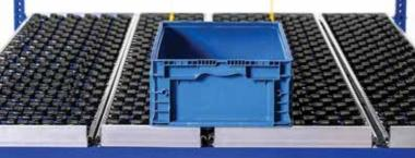
Left: allows loads to overlap lanes and still easily flow for versatile storage
