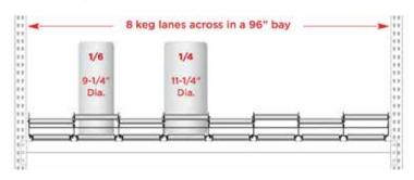
Beer keg storage is difficult: kegs are heavy, difficult to grip, unbalanced and shaped awkwardly—increasing the risk of drops and tip-overs. When the first keg is pulled, the second flows into its place for first-in, first-out stock rotation. With labeled storage lanes, you can slot one keg type per lane to increase organization and picking accuracy.
