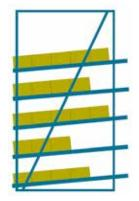
Straight (zero layback) configurations are best suited for full case picking and offer the densest use of floor space. Use when picking full cases such as canned goods or wine.
