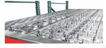
Skatewheels are frequently used in manufacturing and "full shelf" configurations where capacity and product flow are desired. Although configured in lanes, a skatewheel shelf can allow products of many widths and sizes to flow from back to front. A somewhat expensive but very durable option that can be configured to multiple widths.
