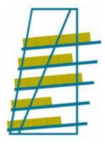
Layback configurations allow access into cartons for split case (each) picking. This requires an extra 1' floor space. Use these to pick from open cases that vary in size.
