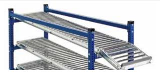
Ideal for cartons, totes or variable size loads. If your carton is less than 6" in width or length, rollers ensure it will flow. Rollers tend to be costlier than wheels, but do not allow fall-through and are less prone to jams. Rollers are also good for round or other irregular load shapes.
