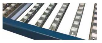
Flow rails use 7/8" wheels on 1.5" centers. Downward facing configuration makes it resistant to collected debris while its galvanized finish resists rust and wear. Use flow rail when the average order consists of multiple items, but only a few pieces per item. The rack should be deep enough to hold a 3-5 day supply of the average item.
