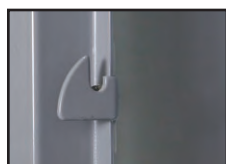
Main door latch hooks welded to frame
