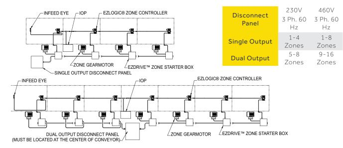
Note: Infeed Wake-Up Eye used only on terminating infeed end of conveyor. Not used when connecting to upstream EZLogic<sup>®</sup> conveyor through power supply isolation cable.
